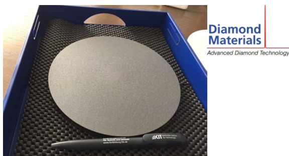
Figure 4. Schematic of the envisaged diamond window brazed in the waveguide at the Brewster angle (top) and picture of the first produced, worldwide, CVD diamond wafer of 180 mm diameter and of 0.3 to 0.45 mm thickness on the substrate (bottom).
