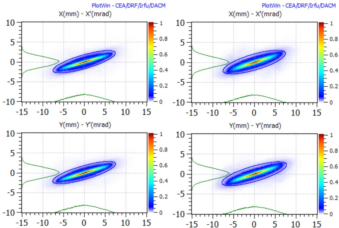
Fig. 8. X-direction (up) and Y-direction (bottom) particles distribution (position vs. angle chart) – calculation with TraceWin (left) and with GPT (right).
