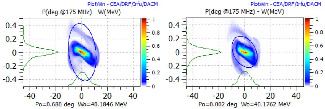
Fig. 9. Phase vs. energy distribution. Left: TraceWin calculation, right: GPT calculation.
