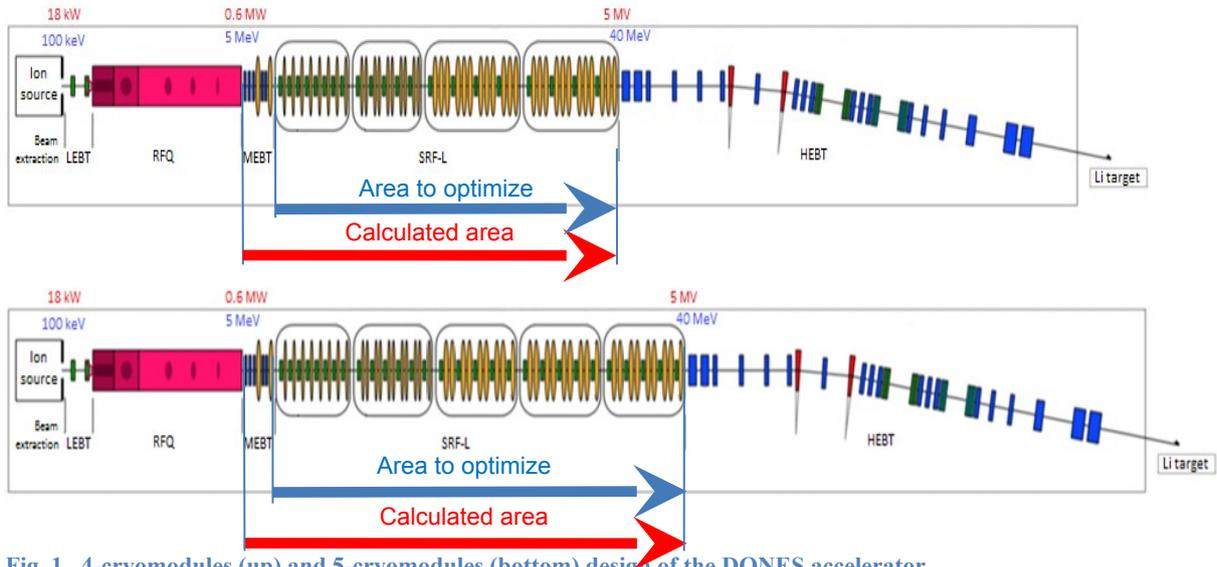
Fig. 1. 4-cryomodules (up) and 5-cryomodules (bottom) design of the DONES accelerator.
