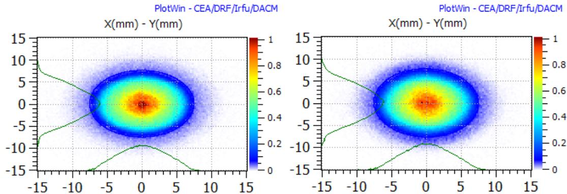
Fig. 7. Geometrical particles distribution in the entrance to HEBT - TraceWin (left) and GPT (right) calculation.
