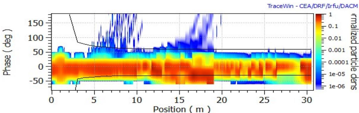
Fig. 6. Density of phase deviation of the beam across the calculated area.
