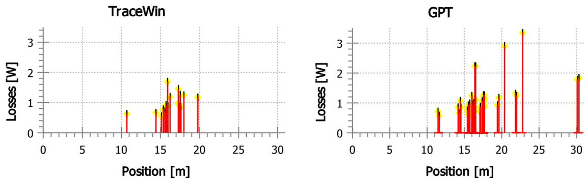
Fig. 2. Total losses for best variant (left: TraceWin calculation; right: GPT calculation).
