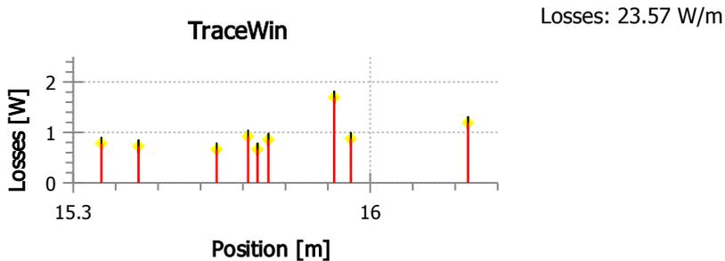
Fig. 3. Losses for the best variant in the worst 1 m long sector calculated with TraceWin (left) and with GPT (right).
