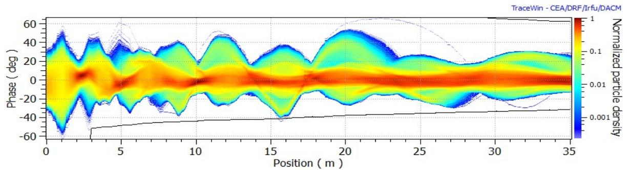
Fig. 12. Density of phase deviation of the beam across the calculated area.
