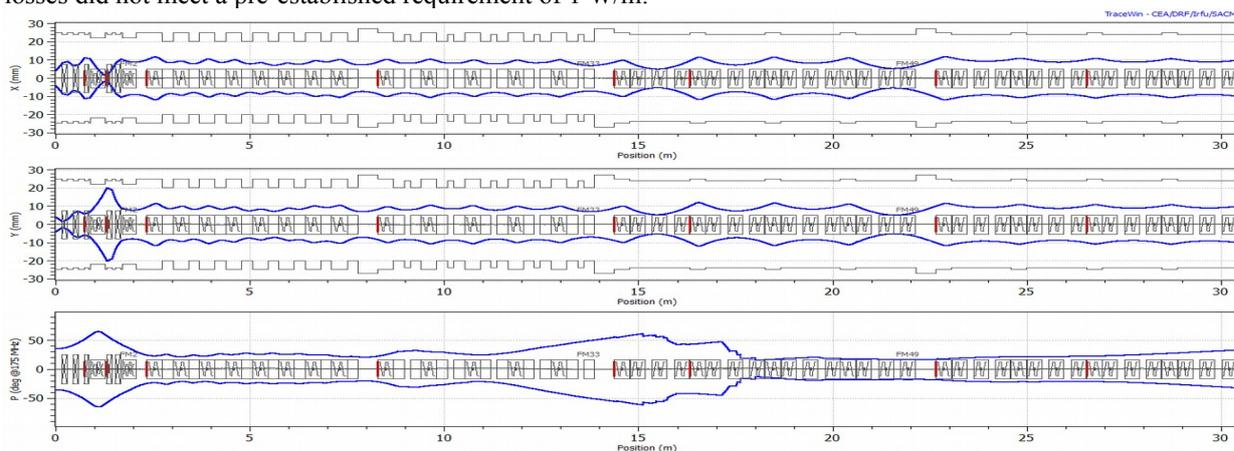
Fig. 4. Envelope of the beam. Top: envelope in X direction; middle: envelope in Y direction; bottom: phase envelope.
