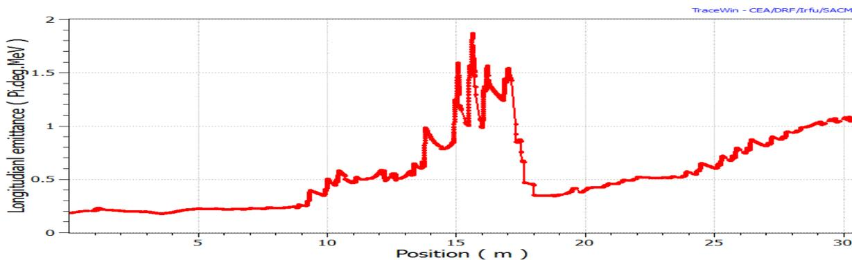
Fig. 5. Longitudinal emittance of the beam across the calculated area.
