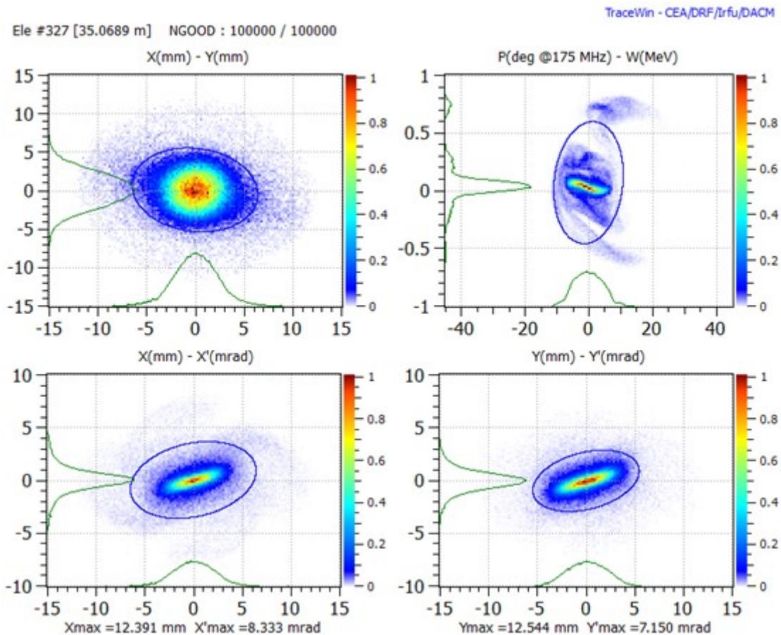
Fig. 13. Deuterons distributions in the exit of the accelerator obtained with TraceWin code. Top left: X-Y distribution; top right: phase vs. energy distribution; bottom: X-direction (left) and Y-direction (right) particle distribution (position vs. angle chart).
