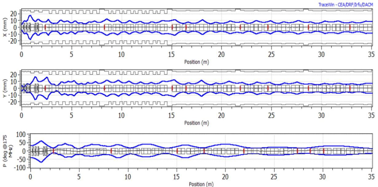
Fig. 10. Envelope of the beam. Top: envelope in X direction; middle: envelope in Y direction; bottom: phase envelope.
