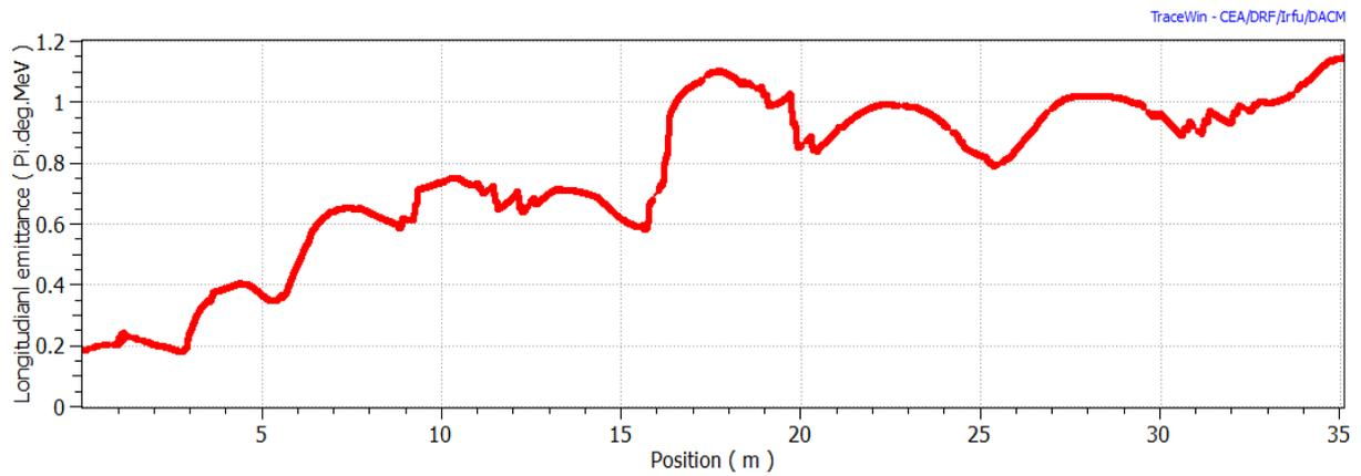
Fig. 11. Longitudinal emittance of the beam across the calculated area.
