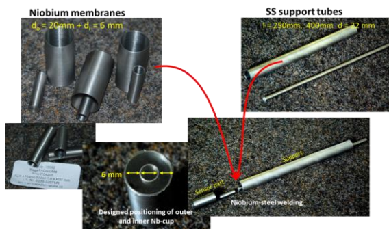
Fig. 4. Dimensions and positioning of niobium cell cups. The Nb-crucibles have diameter of 6 and 20 mm, respectively.
