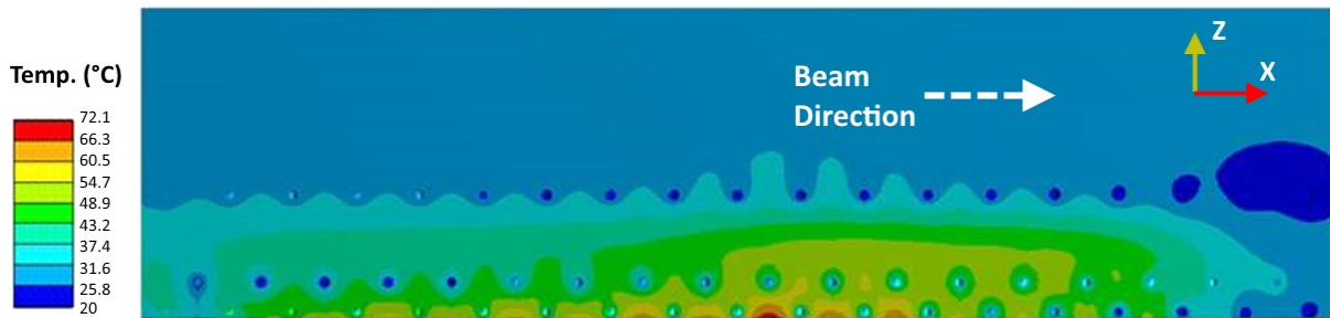
Fig. 4. Temperature map of LSP under helium active cooling condition in the vertical cross-section in the beam direction
