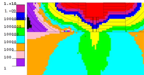
Fig. 6. Neutron flux (n/cm 2 /s) around the Li outlet pipe in the QT half-buried in TC floor lay out during the beam operation (10mm void fraction in the chute) [9].
