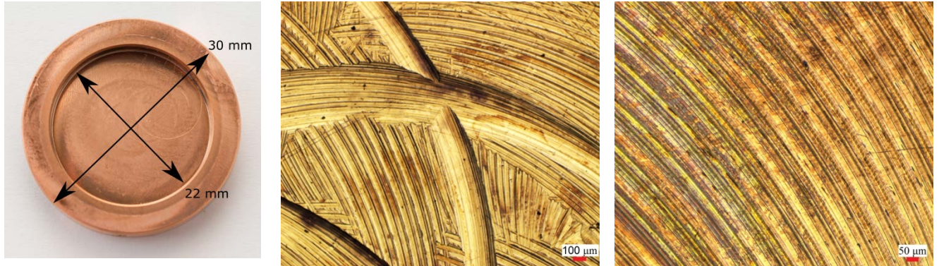
Figure 2: Copper sample photograph and optical microscope images of its surface.
