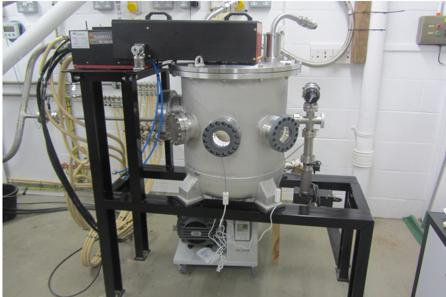
Figure 2: The HIVE vacuum vessel
