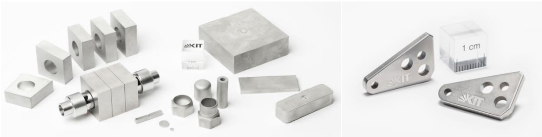
Figure 2. Range of dimension of the produced W-PIM parts (left side) [9]; W-PIM Langmuir probes for WEST (right side) [10]
