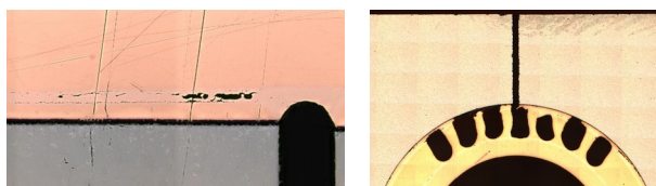
a. Defects in the braze joint at the bottom of mock-up No 6. b. Degradation of spokes in the interlayer, mock-up No 5.
