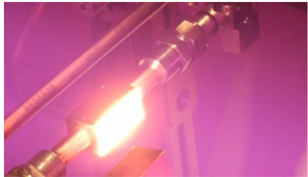
Fig. 1: Arrangement of the mock-ups in GLADIS. The image shows a DEMO type mockup with 12 W blocks at 20 MW/m 2 loading. The mock-ups were fully loaded in the neutral beam. The water connectors are protected by beam scrapers. The scraper of the water outlet (lower left in the image) is visible.
