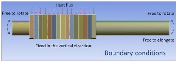
Figure 1. Boundary conditions for FEA calculations
