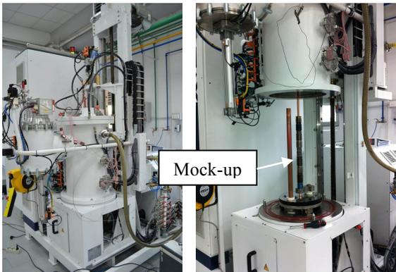
Figure 5 - New DEMO-HRP equipment during mock-up assembly
