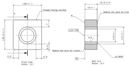
Figure 3 – W block drawing with 12 mm axial thickness
