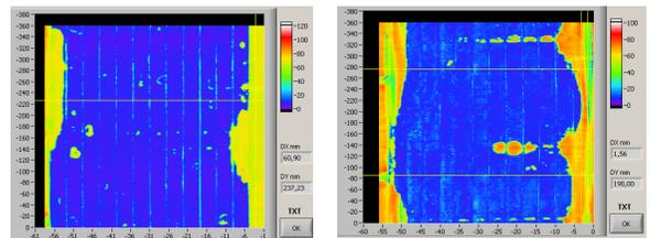
Figure 8: UT C-scans results for #007 and #008 mockups
