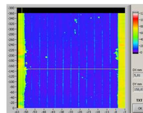
Figure 9: UT C-scan results for #005 mockup
