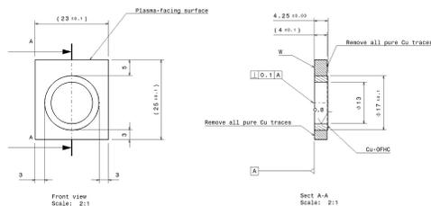
Figure 2 – W block drawing with 4 mm axial thickness
