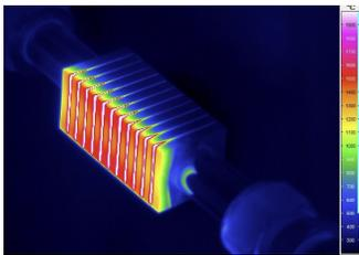
Figure 10: Mock-up #005 - 100th cycle at 20 MW/m<sup>2</sup> loading, water cooling 130°C
