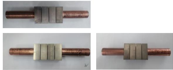
Figure 7 - Picture of the three mock-ups named ITER-like #009, #011 and #012 with 12 mm thickness W blocks.
