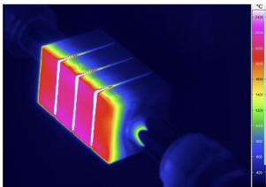
Figure 11: Mock-up #011 - 100th cycle at 20 MW/m<sup>2</sup> loading, water cooling 130°C
