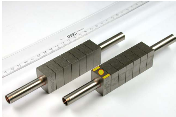
Fig. 1: Examples of ITER W monoblock mock-ups HHF tested in GLADIS. Seven monoblocks of 23 x 28 x 12 mm 3 are bonded onto a cooling tube made of CuCrZr. For one W monoblock, the ROIs for the IR analysis are marked in yellow.
