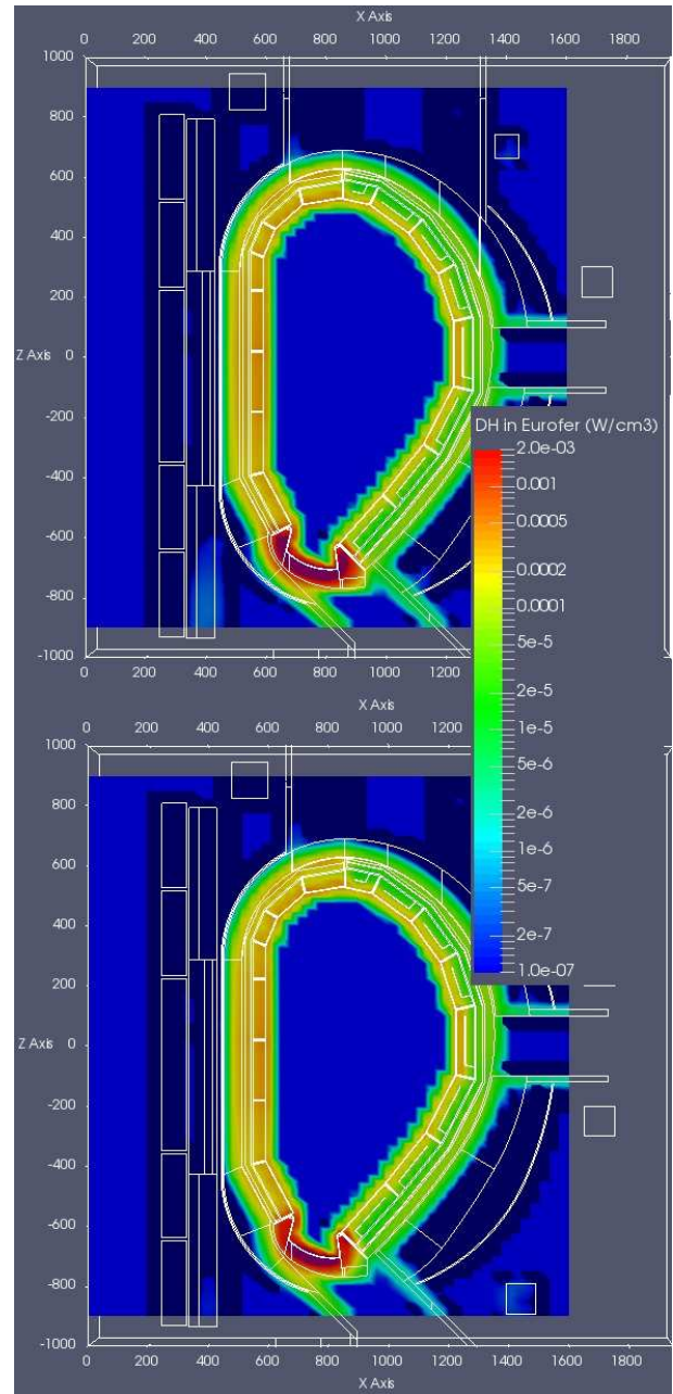
Figure 18: Decay gamma heating in Eurofer at 12 days after shutdown for the DCLL DEMO model with divertor #2 (up) and #3 (down). Values outside the adopted scale are in deep-blue and deep-purple colours.
