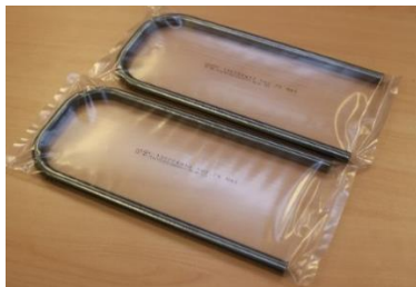
Figure 11: grade 91 bended needle supplied for back plate welding demonstration
