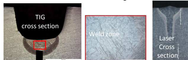
Figure 3: cross sections of TIG and laser welds
