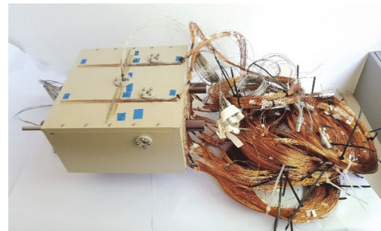
Figure 7 Instrumented WCLL mockup with copper cables and thermocouples.
