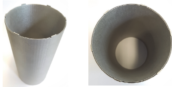
Figure 13: Circular thin-and double-walled FCI mockup with 200mm length and a total wall thickness of 1.5mm. Walls and gap have a thickness of 0.5mm each. The aim was to create straight parts similar to those produced with conventional methods by SLM. Result was a straight part with constant distance and good resolution of the circular shape. The circular shape could be further smoothed by with improved parameters.
