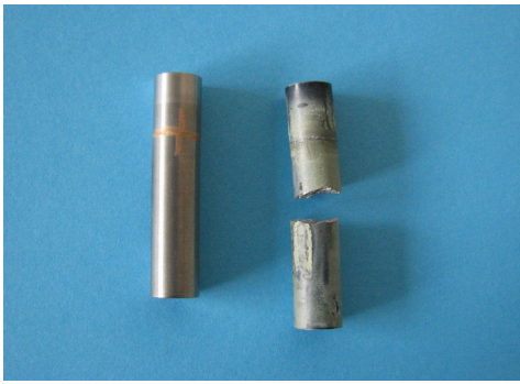
Fig. 2: Electroplating assisted brazing of two tungsten parts, by electroplating of Cu and Ni layers as brazing fillers on W parts: Joined W parts after brazing (left) and after shear testing (right).
