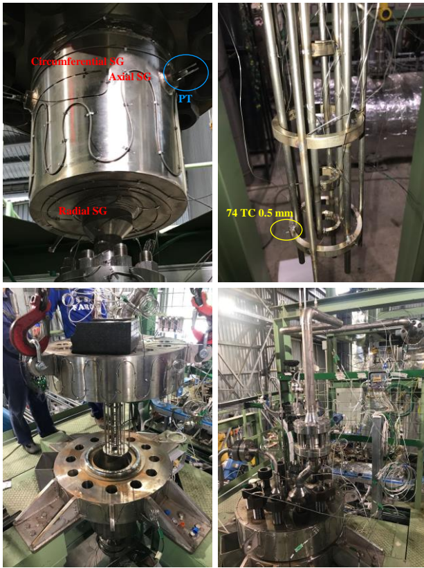
Fig. 4. Test section assembly and instrumentation
