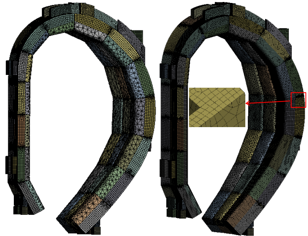
Fig. 6. Coarse and refined mesh of global model.
