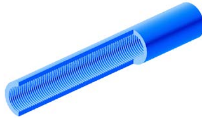
FIG. 1. Geometry of screw tube showing internal thread.
