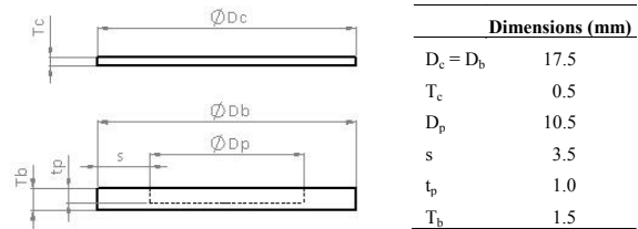
Fig. 2. Schematic and dimensions of the prototype detectors used at the FNG experiment
