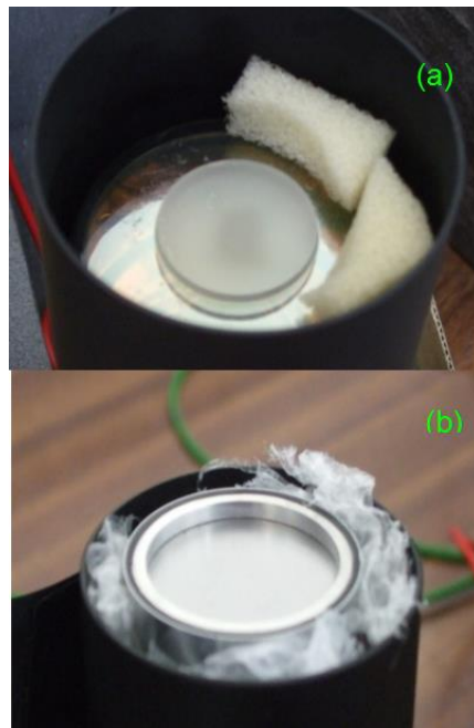
Fig.1 Pictures of thin \text{YAP}:\text{Ce} (a) and \text{LaBr}_3:\text{Ce} (b) crystals coupled to PMTs and used in the measurements described in the text
