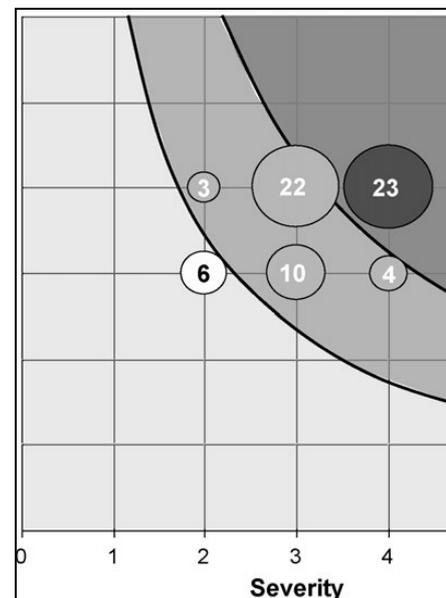
Fig. 7. Initial criticality chart for the ITER TCWS. Numbers and size of circles represent the number of failure modes identified for each set of coordinates: severity and frequency of
