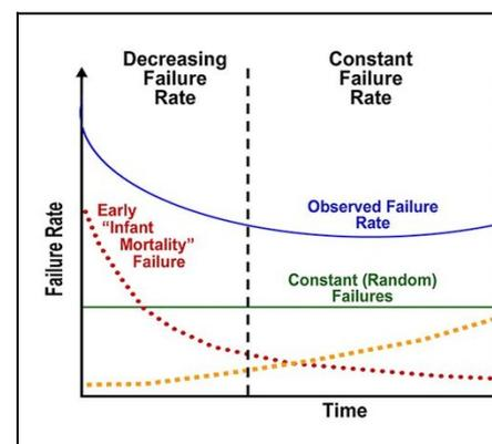
Fig. 1. The bathtub curve, summarizing the three main causes of failure in many components and systems.
