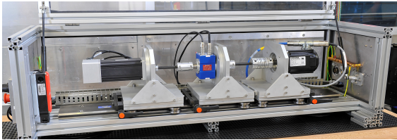
FIG. 4: The actuator test rig used for performance measurements during the development process.
