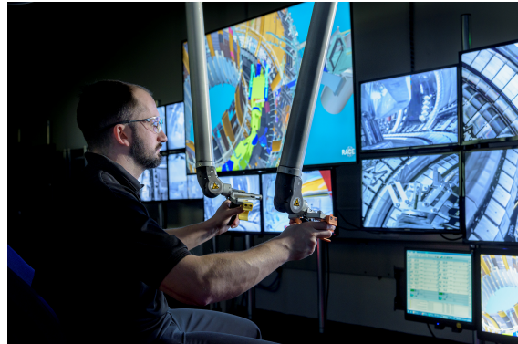
FIG. 1: The mascot master being used to replace components within the JET tokamak.
