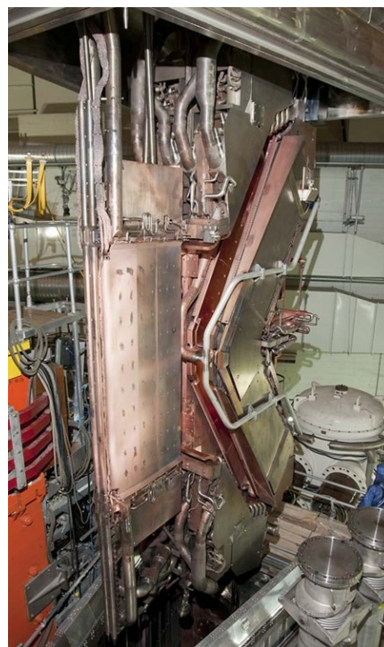
Fig. 2. Neutral beam components being lifted, calorimeter is the tall copper panel on the left.
