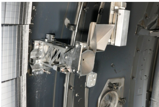
Figure 4. ITER First Mirror installed in JET
