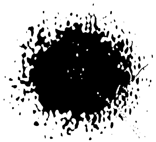
Fig. 2: Burn pattern produced by the injected beam before the torus window. The granular structure is due to reflections from a ceramic load placed between the thermosensitive paper and the window.
