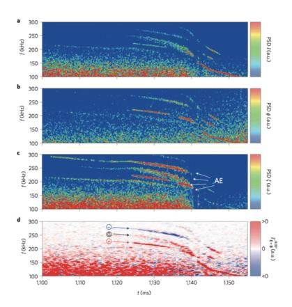
Fig. 5 Observation of AEs in the TJ-II stellarator and their influence on turbulent driven transport: a/b/c) Time evolution of the power spectral densities (PSD) measured at mid-radius for total secondary beam current a), plasma potential b) toroidal shift c). The frequency resolved turbulent particle flux shows outward (red / d) and inward fluxes (blue / d) [54].
