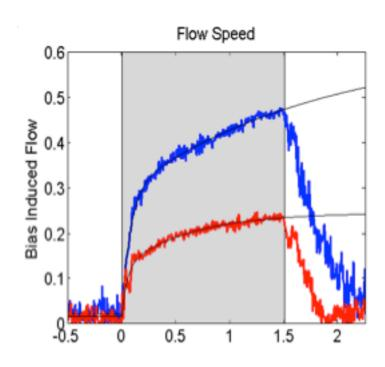
FIG. 1 HSX has direction of symmetry in |B|, hence a direction of minimal flow damping: blue (QHS), red (Mirror) [6]
