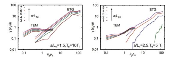
Fig. 3 Linear growth rates of TEM and ETG modes in HSX [37], showing that TEM is only weakly dependent on the temperature gradient and is primarily driven by the density gradient.
