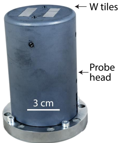
Figure 2: Samples installed in the manipulator before exposure to He-ICWC
