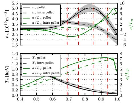
Figure 1: Profiles of density and temperature. Dashed lines indicate radial positions of the NL analysis.
