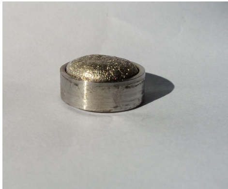
Figure 1: Tin sample in its holder after exposure to ISTTOK plasmas.
