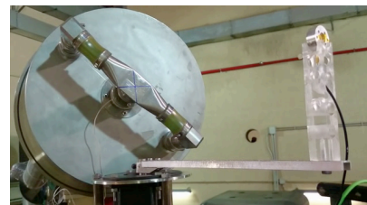
Fig. 4. The diamond detector attached to the arm of the step motor in front of FNG neutron target.
