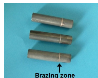
Fig. 3. Brazed samples for thermal treatments and shear testing.
