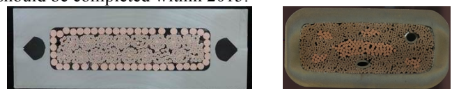
Fig.4 Cross-sections of the two samples: RW1 (left) as prepared for jacketing tests, and WR1 sample (right). The RW1 copper cores and spirals-in-petals (6.6 mm diameter before compaction) are clearly visible.
