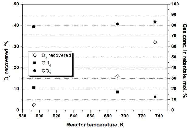
Fig. 7.  $D_{2, recovered}$  values and retentate composition for the WGS tests at different reactor temperature ( $D_2O_{in}=10 \text{ g h}^{-1}$ ,  $D_2O/CO=1$ ,  $p_{lumen}$  of 100 kPa).
