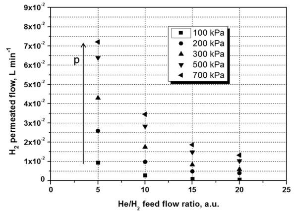
Fig. 2. Hydrogen permeated flow for tests at 623 K (lumen pressure few kPa).
