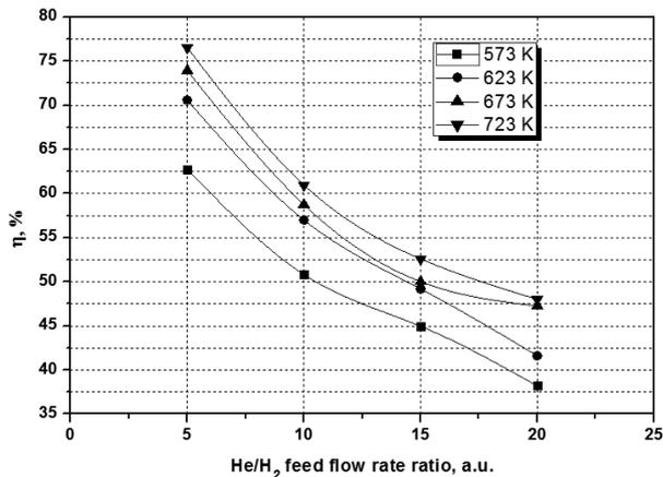
Fig. 5. Efficiency ( $\eta$ ) of hydrogen removal tests along He/H<sub>2</sub> feed flow ratios for several reactor temperature at lumen pressure of 500 kPa (lumen pressure at about few kPa).
