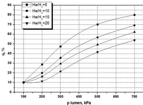
Fig. 4. Efficiency ( $\eta$ ) of hydrogen removal tests along lumen pressure for several He/H<sub>2</sub> feed flow rate ratio at reactor temperature of 623 K (lumen pressure at about few kPa).
