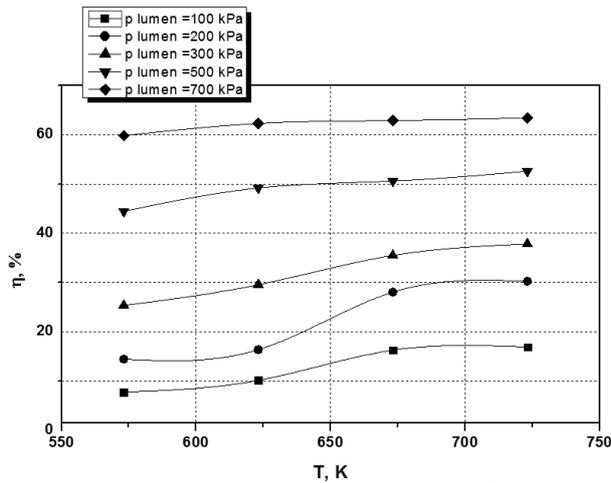
Fig. 3. Efficiency ( $\eta$ ) of hydrogen removal tests for the He/H<sub>2</sub> feed flow rate ratio of 15 (lumen pressure at about few kPa).
