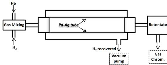
Fig. 1. Block diagram of the experimental set-up of hydrogen recovery tests.
