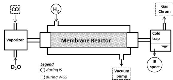
Fig. 6. Block diagram of the experimental set-up used for IS and WGS tests.
