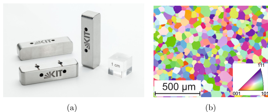
Figure 9: W-PIM parts produced for a study of plasma-wall interaction in ASDEX upgrade (a), EBSD image of the uniaxial grain orientation (b).
