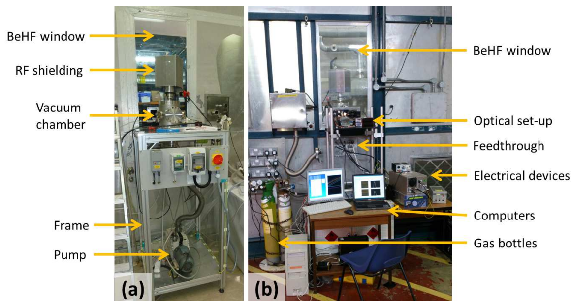
Figure 1: (a) Picture of the vacuum chamber installed inside the JET-BeHF in front of a window and of (b) the equipment needed to control the experiments located outside of the JET-BeHF.
