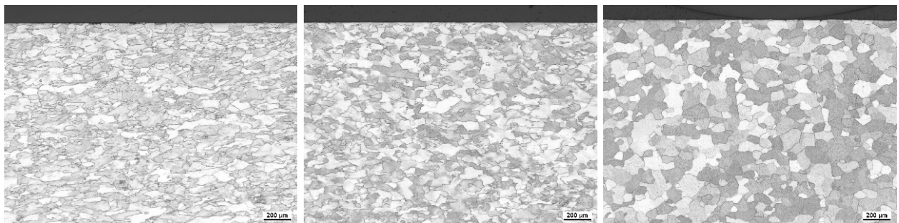
Figure 4. From left to right, the cross-section of the S-, M-, and L-samples with H-exposure after HFF-12 pulses at a base temperature of 1000°C.
