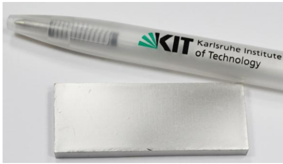
59 Figure 1: Finished plate with dimensions of 55 \times 22 \times 4 \text{ mm}^3 and a weight of \sim 75 \text{ g} ; average tungsten 60 grain size of the produced PIM-W materials.
