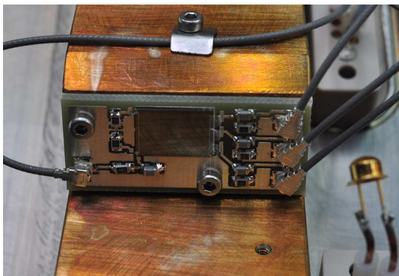
Figure 5: A 5\ \mu\text{m} detector mounted on a PCB as installed on KF1 vacuum flange prior to installation on the machine. Hirose U-FL-series ultra-miniature connectors are used for bias (left) and AC-coupled signal connections (right). The detector is read-out as three banks of 20 strips. An IR LED for artificial excitation of the detectors is seen at lower left.
