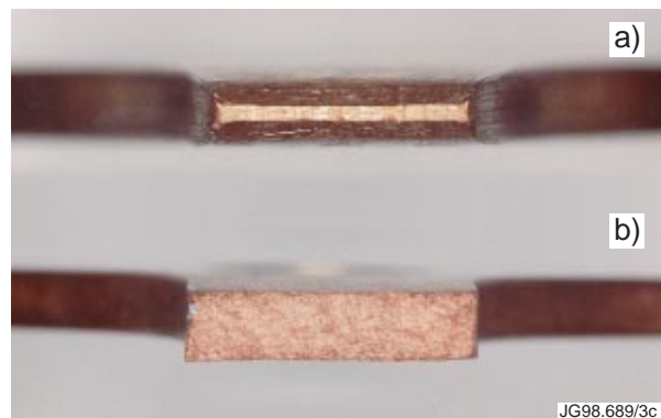
Fig.6. Fracture surface of a) solution and b) precipitation hardened CuNiSi specimens following a room temperature tensile loading.
