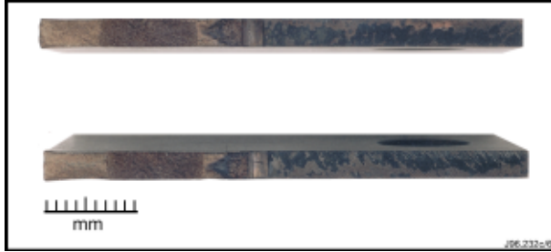
Fig.8. Characteristic triangular shape of a CT fractured surface demonstrated throughout the fracture toughness tests at all temperatures.
