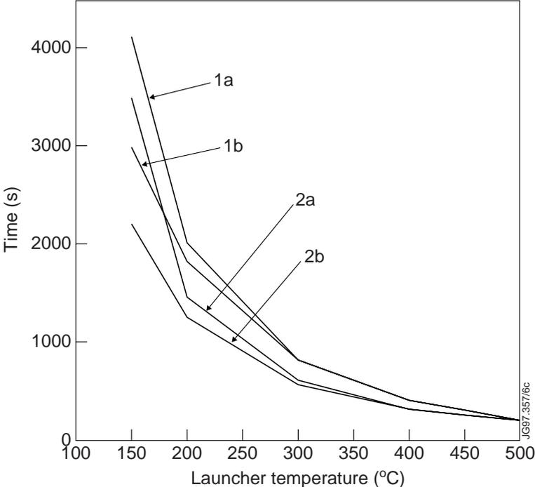
Figure 7. Boiling times of the LHCD flap versus launcher temperature in a hypothetical loss of water flow incident. (For curve labels see text).
