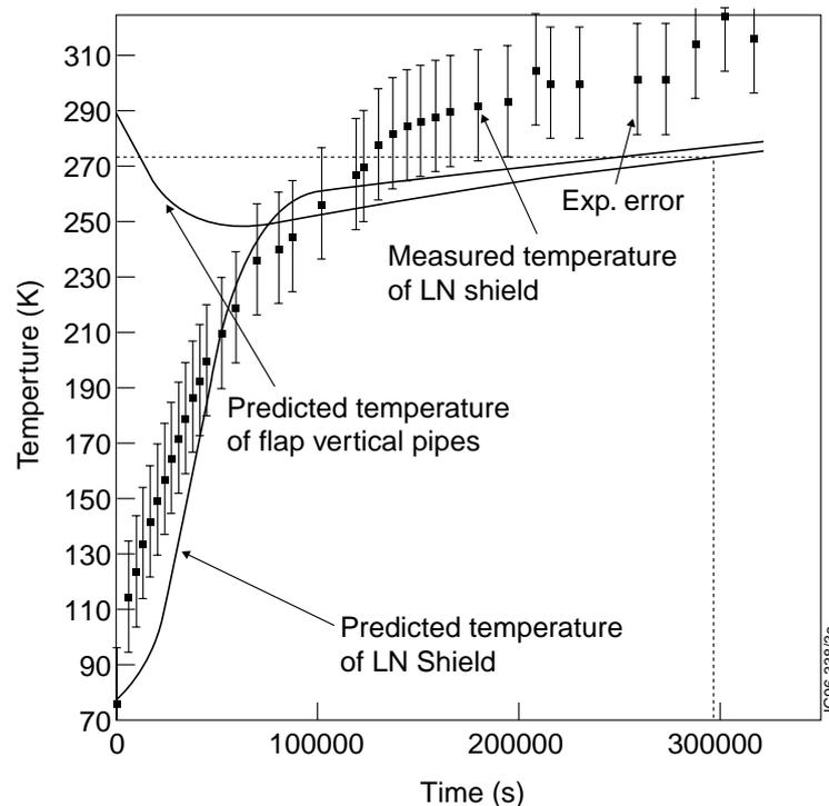
Figure 5. Comparison between model prediction and measurements of the LHCD cryopump system during a freeze-up incident.
