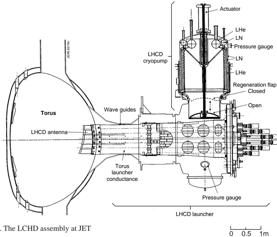
Figure 1. The LHCD assembly at JET
