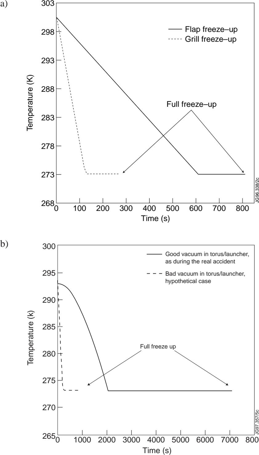
Figure 6. Predicted freeze-up of LHCD components (a) flap and grill of the cryopump (b) flap supply pipes.
