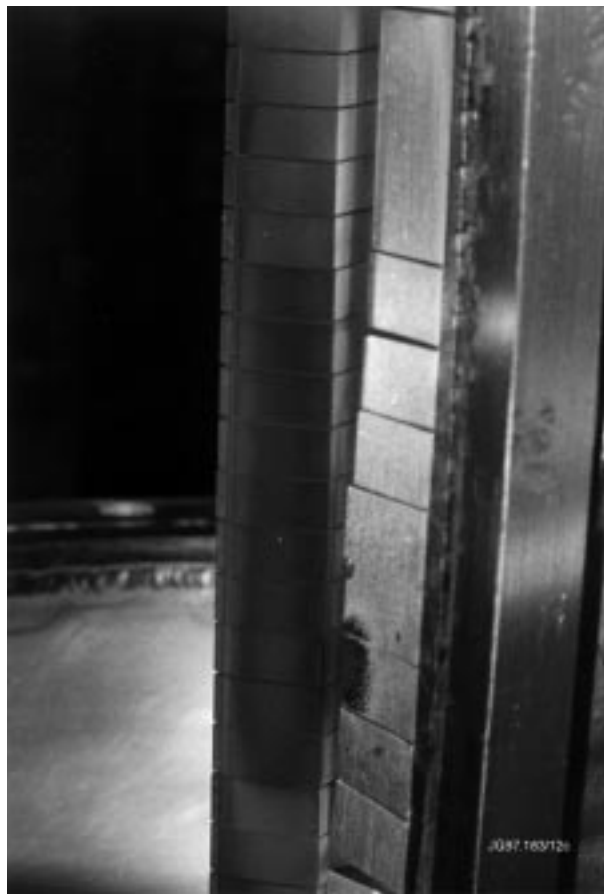
Fig.12: Photographs of the tile after part 1. Left: The discoloration of the Beryllium reflects the intensity of the exposure. The copper calorimeter shows substantial deformation and discoloration - probably Beryllium from previous tests. In this test there was no melting at the time this pictures were taken (end of part 1).
