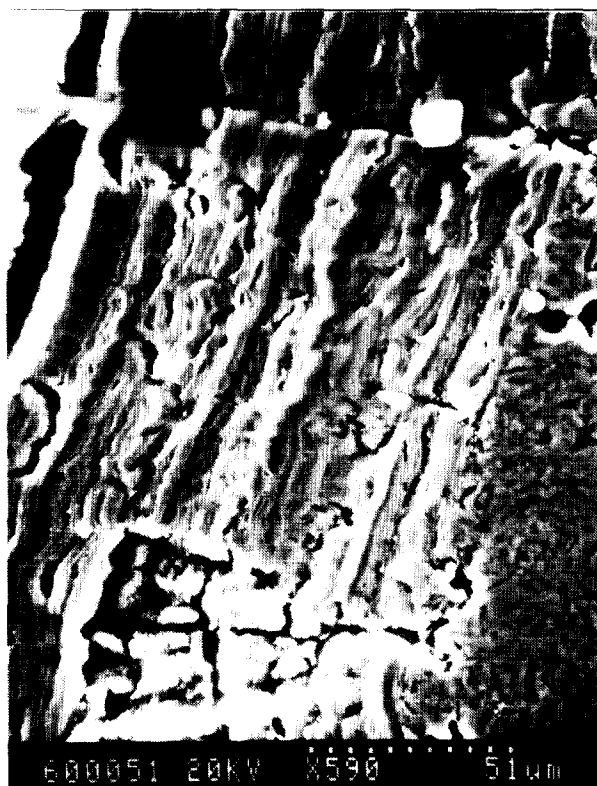
Figure 5. An optical micrograph of a section through a thick redeposited layer on the side of a 1986 JET limiter. Layers deposited in each period of the operations can still be distinguished.
