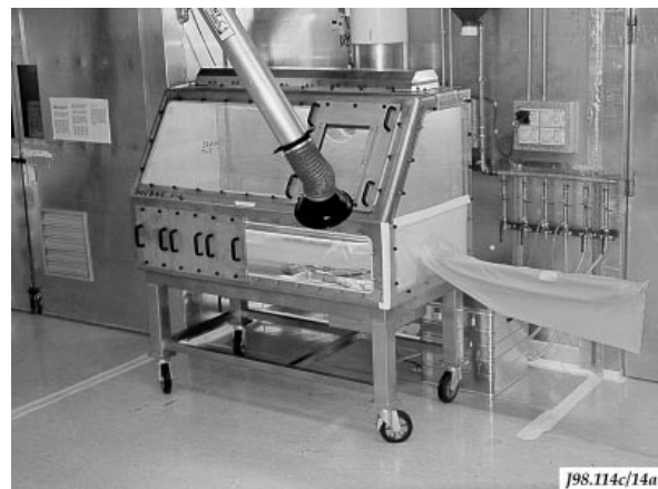
Fig.4: Ventilated enclosure in fume cupboard mode
