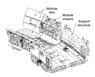
Figure 4 JET MkIIa Divertor construction
