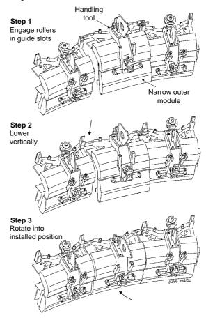
Figure 8 Installation sequence for divertor modules
