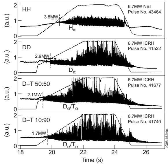
FIG. 14.  $D_\alpha$ -signal and input power plotted as a function of time in four shots with different gas mixtures: hydrogen, deuterium, 50:50 D:T and 10:90 D:T. Same input power (6.7 MW) with a slow ramp was used to identify the onset of H-mode at the first appearance of ELMs as indicated. Threshold power decreases with increasing isotopic mass.
