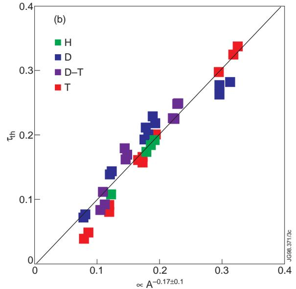
FIG. 17 (b). Core plasma thermal energy confinement time in H-mode discharges is plotted as a function of the gyro-Bohm scaling for JET discharges in different isotopic mixtures of H, D and T.
