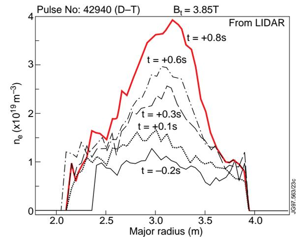
FIG. 9 (b) Electron density profiles measured by LIDAR diagnostics for a number of time slices during an optimised shear discharge in D-T plasmas in JET. The time ( $t$ ) parameter refers to the start of the high power phase.
