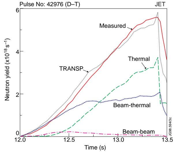
FIG. 5. Time evolution of the observed total neutron yield compared with a provisional simulation (run Y905) from the TRANSP code for the highest (16.1 MW) fusion power output shot of JET shown in Fig. 3. Also shown are the thermal, beam-thermal and beam-beam contributions to the neutron yield as predicted by the code. This simulation is presently undergoing further checks and verifications of ion temperature and effective charge.
