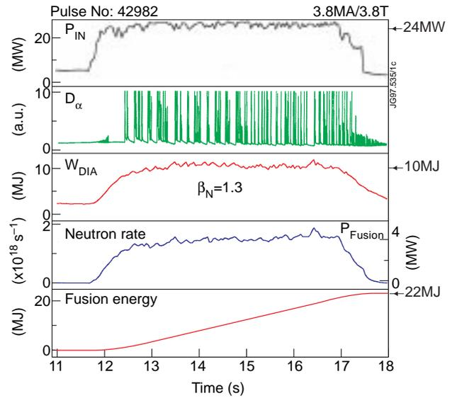
FIG. 6. Time traces of a near steady-state high performance JET discharge at 3.8T/3.8MA in 50:50 D:T mixture with an input power ( $P_{\text{in}}$ ) of 24 MW. Diamagnetic stored energy ( $W_{\text{DIA}}$ ) reached 10.5 MJ, fusion power output ( $P_{\text{FUS}}$ ) and total  $Q$  ( $\equiv P_{\text{FUS}}/P_{\text{in}}$ ) are 4.1 MW and 0.18 respectively. ELMs are shown by the  $D_{\alpha}$ -signal.
