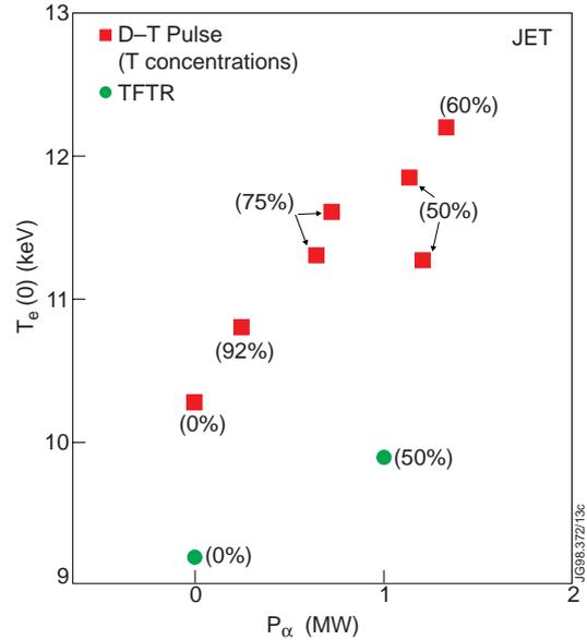
FIG. 12. Central electron temperature versus alpha-particle power in JET D-T discharges where the NBI input power was kept at about 10.5 MW. The numbers in parenthesis show the tritium concentration for this series of discharges. Also, shown are two data points of TFTR for comparison.
