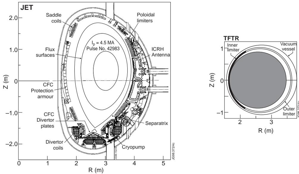
FIG. 1. Poloidal cross sections of JET and TFTR tokamaks. Also, shown are the four divertor coils, MkIIaP divertor target plates, the cryopump, an ICRH antenna, a poloidal limiter and saddle coils inside the JET vacuum vessel. Plasma flux surfaces together with the separatrix of a 4.5 MA discharge are also illustrated.
