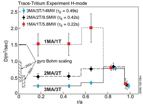
FIG. 21 (b). Profile of particle diffusivity ( $D$ ) derived from JET trace tritium ITER similarity H-mode plasmas in deuterium at 1T/1MA, 2T/2MA and 3T/3MA. Normalized to 1T, the expected band of values at the centre for gyro-Bohm scaling for 2 and 3T are also shown schematically. The shaded bands represent the uncertainty in central  $T_i$  measurements.
