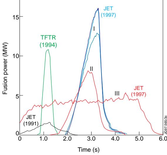
FIG. 10. Fusion power development in the D-T campaigns of JET and TFTR. (I) Hot ion H-modes, (II) Optimized shear and (III) Steady-state ELMy H-modes.
