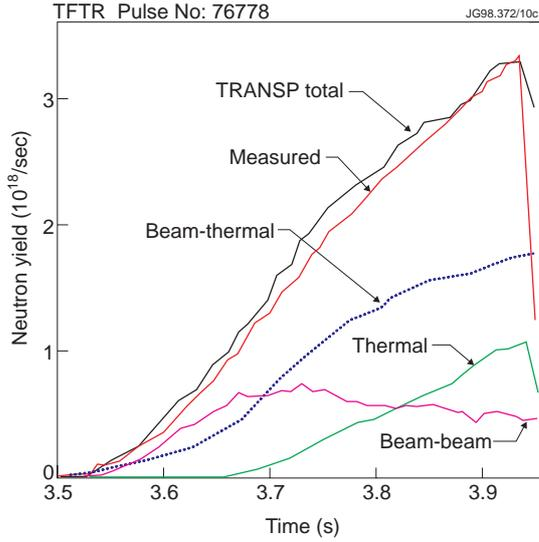
FIG. 4. Time evolution of the observed total neutron yield is compared with a simulation from the TRANSP code for the highest (10.7 MW) fusion power output shot of TFTR. Also shown are the thermal, beam-thermal and beam-beam contributions to the neutron yield as predicted by the code.
