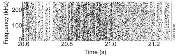
FIG. 18. A contour plot of spectral intensity of the reflectometer phase fluctuations at  $R \sim 2.55\text{ m}$  ( $r/a \sim 0.5$ ) in the frequency-time plane for the JET shot #42808. Note that the intermittent bursts of fluctuations observed in this shot are not correlated either with ELMs, sawteeth or rotating MHD modes.
