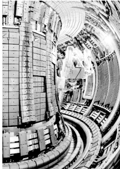
FIG. 23. A photograph of the inside view of the JET tokamak showing the MkII Gas-box divertor on the floor. The divertor tiles were installed by the remote handling tool shown above. Also shown are the ICRH antennae and the LHCD launcher on the right-hand side of the picture.
