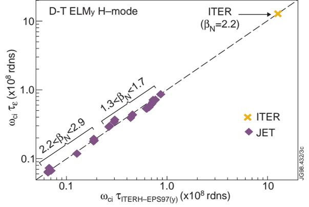
FIG. 11. Thermal energy confinement time data of JET D-T shots in dimensionless form is plotted as a function of the scaling obtained from the gyro-Bohm transport model. The ITER expected value of confinement in D-T plasmas is in line with that extrapolated from the JET D-T data.
