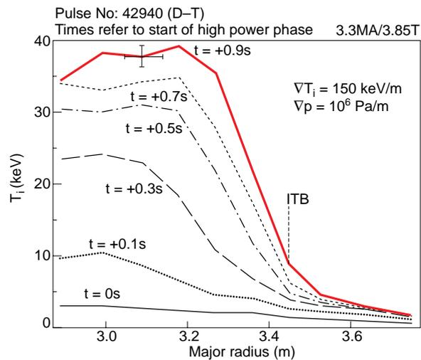
FIG. 9 (a) Ion temperature profiles measured by charge-exchange recombination spectroscopy for a number of time slices during an optimised shear discharge in D-T plasmas in JET. The time ( $t$ ) parameter refers to the start of the high power phase. An internal transport barrier is triggered at  $t=0.3$  s.
