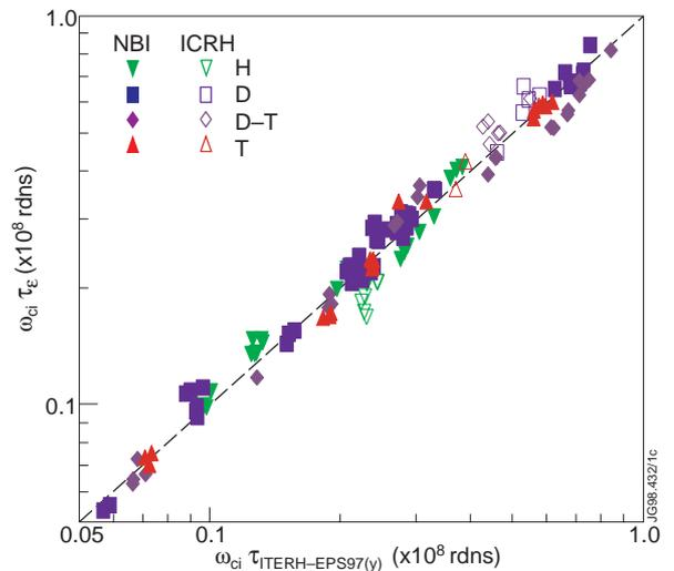
FIG. 16. Thermal energy confinement time is plotted as a function of the normalised ITERH-EPS97y scaling for the JET discharges in D-D, D-T and T-T plasmas heated by ICRH and NBI as indicated.
