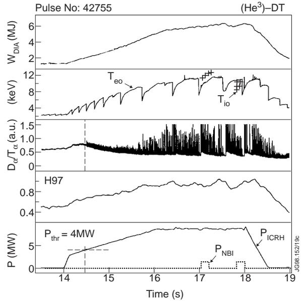
FIG. 22. Time traces of a  $\text{He}^3$ -minority ICRF heating of a 45:55 D:T plasma with about 10% of  $\text{He}^3$  added. Other parameters are  $B_\phi=3.7T$ ,  $I_p=3.3MA$ ,  $f=37.2MHz$ , and  $n_{e0}=3.2 \times 10^{19} m^{-3}$ . Central electron and ion temperatures are 12 and 13 keV respectively. The ITERH97-Py factor is close to unity.
