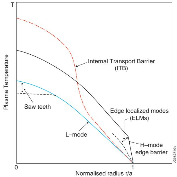
FIG. 2. Tokamak temperature profiles are shown schematically for a number of modes of operation. Sawteeth flatten the central electron temperature profile periodically whereas the ELMs degrade the edge pedestal.
