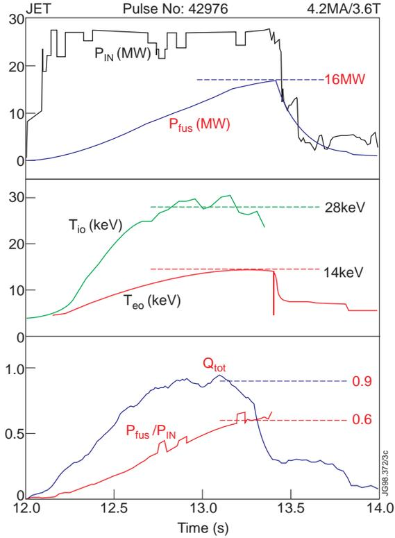
FIG. 3. Time traces of the highest performance JET D-T hot-ion H-mode discharge producing a record fusion power output of 16 MW and a  $Q = P_{\text{fus}}/P_{\text{in}} = 0.62$ .
