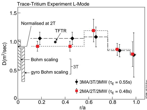
FIG. 21 (a). Profile of particle diffusivity ( $D$ ) derived from JET trace tritium ITER similarity L-mode plasmas in deuterium at 2T/2MA and 3T/3MA. Normalised to 2T data, the expected band of values at the centre for Bohm and gyro-Bohm scalings for 3T are also shown schematically. The shaded bands represent the uncertainty in central  $T_i$  measurements.
