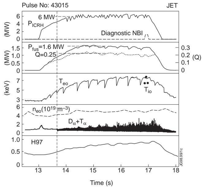
FIG. 7. Time traces of a near steady-state JET discharge at 3.8T/3.8MA in 9:91 D:T mixture heated by ICRH in D-minority in tritium with an input power of 6 MW. Fusion power output is 1.6 MW making a record  $Q=0.22$  for a duration of more than 2.5 s. Here, H97 represents the ITERH97-Py H-mode confinement factor which is above the value required by ITER.
