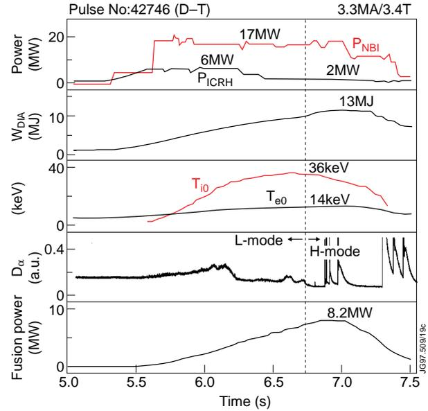
FIG. 8. Time traces of an optimised shear discharge in JET where the fusion power output reached 8.2 MW. The performance degrades at the appearance of ELMs. Central ion and electron temperatures reached 36 and 14 keV respectively.
