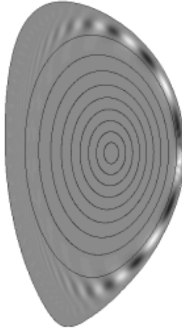
Fig.13b The displacement due to an n=10 ballooning mode. Red and Blue represent the minima and maxima of the displacement.
