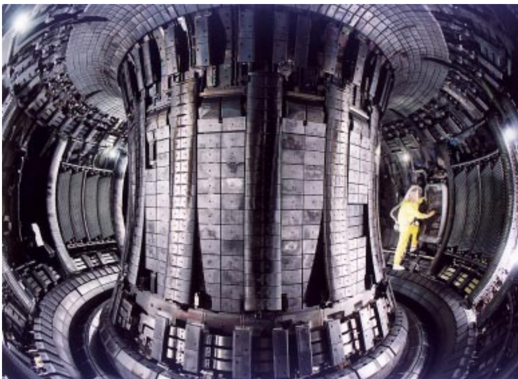
FIG. 1. A view of the in-vessel components of JET (1997) with MkIIa divertor on the floor of the torus. On the right hand side, an array of 4 ICRH antennas adjacent to the LHCD launcher and a poloidal limiter can be seen.
