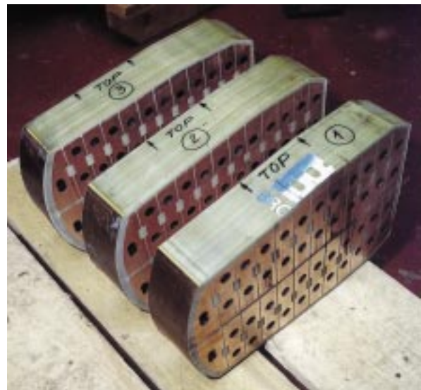
Fig. 6. Cuts of one of the replaced toroidal coils for visual inspection and for extracting test samples
